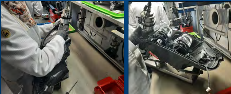
ULTRASONIC CUTTING to access to the subcomponents
